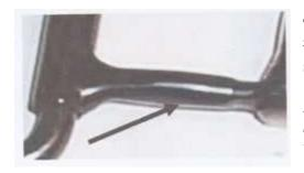
The mouthpiece will consist of a metal bar 5/16" to <sup>3</sup>/<sub>4</sub>" in diameter, as measured 1 inch in from the shank.
